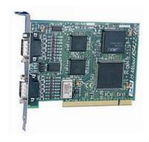
This half size card can run at an amazing speed of up to 18,000,000 baud. It provides 2 industry standard RS422/485 serial ports for PC compatibles in a single PCI slot. The card has on-board zener diodes giving transient spike protection to the inputs - making it ideal for factory automation installations.
