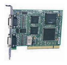
This half size card can run at an amazing speed of up to 15,000,000 baud. It provides 2 industry standard RS422/485 serial ports for PC compatibles in a single PCI slot. The card has on-board zener diodes giving transient spike protection to the inputs - making it ideal for factory automation installations.
