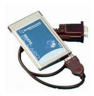
A PCMCIA type II card providing a single RS232 serial port. The megabaud transfer rates and the 128 byte deep FiFO, coupled with the 1Mbit/s line drivers deliver uncompromising performance on your desktop PC. Being mobile no longer limits your options.
