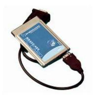
A PCMCIA type II card providing a single serial port configurable as RS422 or RS485 full or half duplex. The megabaud data transfer rates and the 128 byte deep FIFO, coupled with the RS485 Half Duplex Hardware Implemented Autogating guarantees uncompromising performance and fault-free use for the laptop user. Baud rates are software selectable.
