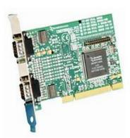
This half size card provides 2 industry standard 9 pin RS232 serial COM ports in a single PCI slot and 1 LPT port. By adding the optional LPT Adaptor cable, a parallel printer port becomes available. As PCI is fully Plug and Play compatible the operating system or BIOS automatically configures card ensuring conflict free installation.
