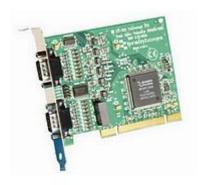
Optical isolation provides greater protection from electrical current surges to both the card itself and the PC. It improves noise immunity by isolating the PC from the card's transmit ground. Opto-Isolation: 1500Volt DC/ 1000Volts AC. Two serial ports independently configurable as RS422 with and without hand-shaking, or RS485 full or half duplex.
