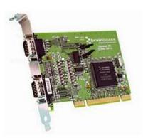
\* RS422/485 Options: RS422: Automatic CTS/RTS flow control, software enabled RS485 -Automatic Hardware half duplex RS485 Gating 485 FEATURES: RxD-/TxD- multiplex jumpers Wiring Schemes: One talker, many listeners Many talkers/listeners full dup
