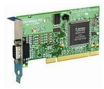
\* Greater control of FIFO trigger levels, and readable FIFO levels for improved transfer efficiency
