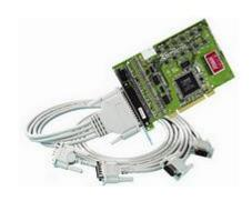
Brainboxes UC-368 Universal PCI 4 Port OPTO Velocity RS422/485 provides four serial ports independently configurable as RS422 with and without hand-shaking, or RS485 full or half duplex, with opto isolation on all RS422/485 lines. The card has on-board zener diodes giving transient spike protection to the inputs, making these cards ideal for factory automation installations.
