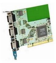
This card provides three industry standard 9-pin RS232 serial COM ports using just a single PCI slot. As PCI is fully Plug and Play compatible, the operating system or BIOS automatically configures the card ensuring conflict free installation.
