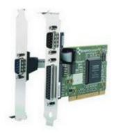
This card provides an LPT parallel printer port and an industry standard RS232 serial COM port. The LPT parallel printer port uses the standard 25 pin female 'D' connector, whilst the RS232 port uses the standard 9 pin male 'D' connector. A second serial COM port is available on the flying lead header using the optional male 9 pin 'D' type serial cable. As PCI is fully Plug and Play compatible, the operating system or BIOS automatically configures the card ensuring conflict free installation.
