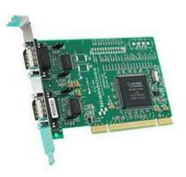
The PCI Dual RS232 POS card is a powered 2 port card, ideal for connecting and powering peripherals such as bar code readers, printers, card readers, display units and cash drawers. Both UP-880 and UP-869 are selectable power options. Ground or 12V can be selected on pin 1 of each port and also 12V or 5V can be selected on pin 9 of each port.
