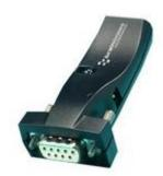
On the hardware front Brainboxes have developed a new Bluetooth serial port adaptor to enable 'dumb' devices with RS232 serial connectors to connect wirelessly with other devices. The compact Brainboxes BL-819 is ideal for printers, scanners and other devices since it brings Bluetooth wireless technology to devices without the need to install any software.
