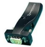
On the hardware front Brainboxes have developed a new Bluetooth serial port adaptor to enable 'dumb' devices with RS232 serial connectors to connect wirelessly with other devices. The compact Brainboxes BL-819 is ideal for printers, scanners and other devices since it brings Bluetooth wireless technology to devices without the need to install any software.
