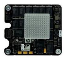
HP Storageworks 160GB I/O Accelerator for BladeSystem c-Class.
