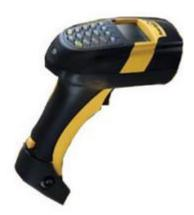
\* Water and particulate sealing rating: IP65/IP64
